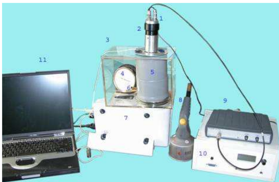
Рис. 4-9-2. UV Photomultiplier 2. EMF shielding cover 3. Main chamber 4. hygrometer 5. Sealed GDV chamber containing electrode; 6. Gas tubes 7. GDV Camera 8. Drier Dryer with silica gel 9. Digital oscilloscope 10. Photomultiplier power source 11. Computer.
